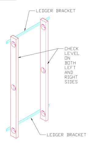
Bubbles on the builder's level must read the same for both vertical sides.
